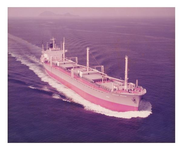
Vessel Name : M.V. Cavalier Bulker Ex-Name : Hitachi newbuilding hull no.4543 When/Where Built : 1977 / Maizuru, Japan Shipyard : Hitachi Shipbuilding and Engineering Co. Ltd. Acquired by Eddie Steamship Group : 1977 Registry : Liberia (Mediterranean International Nav. Corp.) Classification : ABS Length Over-All : 182 meters Breadth : 28 meters GRT/NRT : 20608 / 15065 Deadweight : 36,251 MT (Summer)
