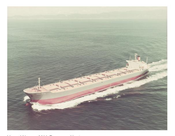
Vessel Name : M.V. Panamax Neptune Ex-Name : MHI newbuilding hull no. 1042 IMO Number : 7314084 When/Where Built : 1973 / Kobe, Japan Shipyard : Mitsubishi Heavy Industries Acquired by Eddie Steamship Group : 1973 Registry : Liberia (Trans Atlantic Marine Corp.) Classification : BV Length Over-All : 233 meters Breadth : 32.2 meters GRT/NRT : 32020 / 22755 Deadweight :61,604 LT (Summer)
