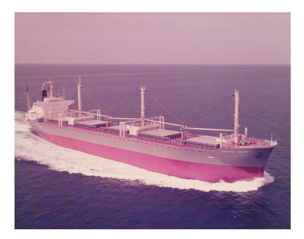
Vessel Name : M.V. Chieftain Bulker Ex-Name : Hitachi newbuilding hull no.4542 IMO Number : 7519024 When/Where Built : 1977 / Maizuru, Japan Shipyard : Hitachi Shipbuilding and Engineering Co. Ltd. Acquired by Eddie Steamship Group : 1977 Registry : Liberia (Pacific International Nav. Corp.) Classification : ABS Length Over-All : 182 meters Breadth : 28 meters GRT/NRT : 20608 / 15065 Deadweight : 36,255 MT (Summer)
