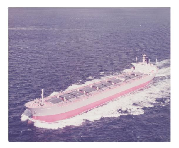
Vessel Name : M.V. Panamax Mercury Ex-Name : MHI newbuilding hull no. 1072 IMO Number : 7527136 When/Where Built : 1977 / Kobe, Japan Shipyard : Mitsubishi Heavy Industry Acquired by Eddie Steamship Group : 1977 Registry : Liberia (Explorer Nav. Corp.) Classification : BV Length Over-All : 238 meters Breadth : 32.2 meters GRT/NRT : 32042 / 22742 Deadweight :61,550 LT (Summer)
