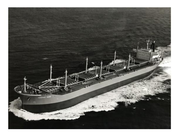
Vessel Name : M.V. Panamax Mars Ex-Name : Hitachi newbuilding hull no. 4519 IMO Number : 7530353 When/Where Built : 1977 / Osaka, Japan Shipyard : Hitachi Shipbuilding and Engineering Acquired by Eddie Steamship Group : 1977 Registry : Liberia (Oriental Oceanic Nav. Corp.) Classification : ABS Length Over-All : 224.468 meters Breadth : 32.2 meters GRT/NRT : 29860 / 22818 Deadweight :60,651 LT (Summer)
