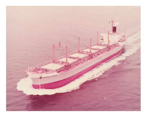
Vessel Name : M.V. Oceanus Countess Ex-Name : MHI newbuilding hull no.1810 IMO Number : 7612711 When/Where Built : 1977 / Japan Shipyard : Mitsubishi Heavy Industries Ltd. Acquired by Eddie Steamship Group : 1977 Registry : Liberia (Kristiansand Marine Co.) Classification : BV Length Over-All : 186 meters Breadth : 27.8 meters GRT/NRT : 21666 / 14287 Deadweight : 39,817 MT (Summer)
