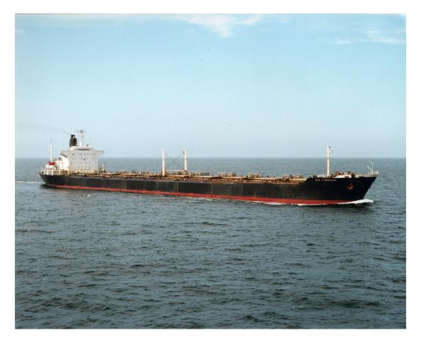
Vessel Name : M.V. Sea Commander Ex-Name : Standard Venture IMO Number : 7112591 When/Where Built : 1971 / Japan Shipyard : I.H.I., Hull No. 2167 Acquired by Eddie Steamship Group : 1987 Registry : Cyprus (Methoni Shipping Co. Ltd.) Classification : ABS Length Over-All : 255 meters Breadth : 32.2 meters GRT/NRT : 37954 / 26846 Deadweight : 71,640 LT (Summer)
