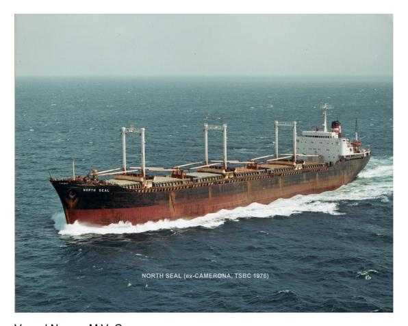
Vessel Name : M.V. Camerona Ex-Name : TSBC newbuilding hull no.057 IMO Number : 7405742 When/Where Built : 1976 / Keelung Shipyard : Taiwan Shipbuilding Corp. Acquired by Eddie Steamship Group : 1976 Registry : Liberia (Continental Oceanic Nav. Corp.) Classification : ABS Length Over-All : 181 meters Breadth : 25 meters GRT/NRT : 17894 / 11779
