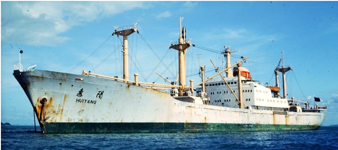
HUI YANG had a particularly sturdily plated signal/radar mast between bridge and funnel (coll. SK).
