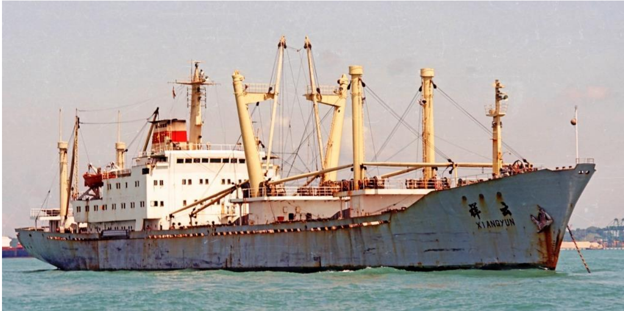
XIANG YUN 30-ton Stülcken evidently reconfigured with two lighter derricks at Singapore May 1992 (Martin Klingsick/shipping.com).
