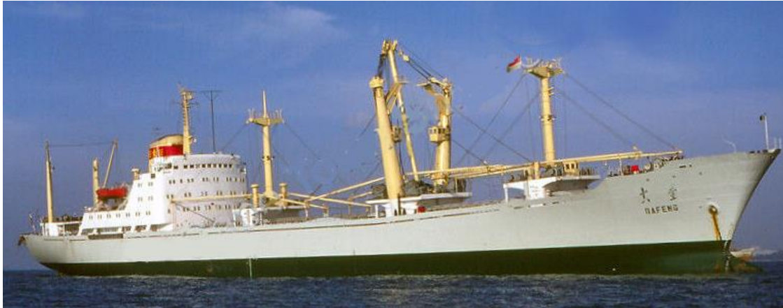
DA FENG with 120-ton Stülcken derrick (Internet).
