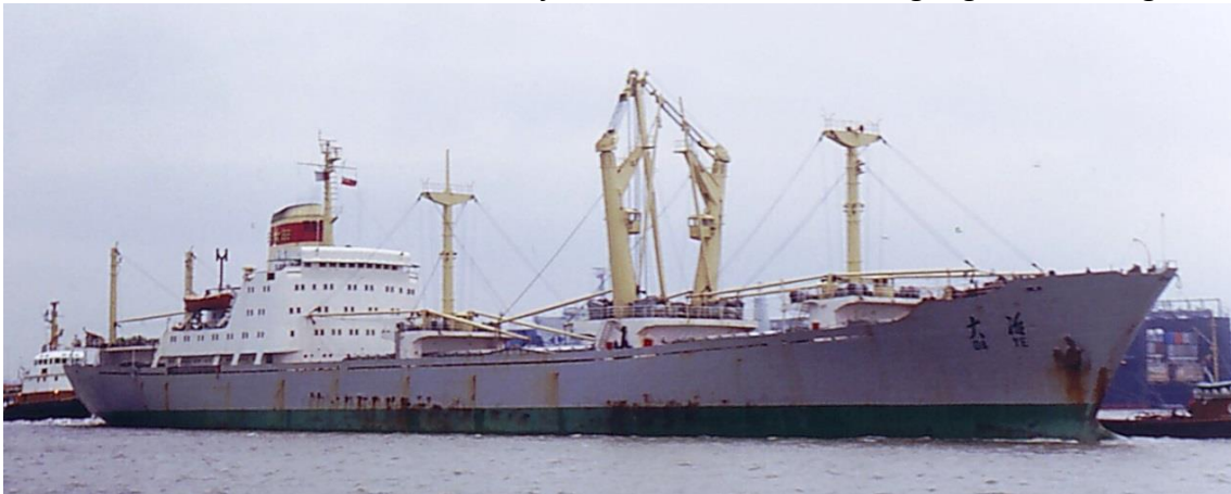
DA YE inbound at Tilbury, 17 October 1981. New formulation of four hatches forward, long No.3 hatch and Stülcken heavylift derrick (John Jones/shipping.com).
