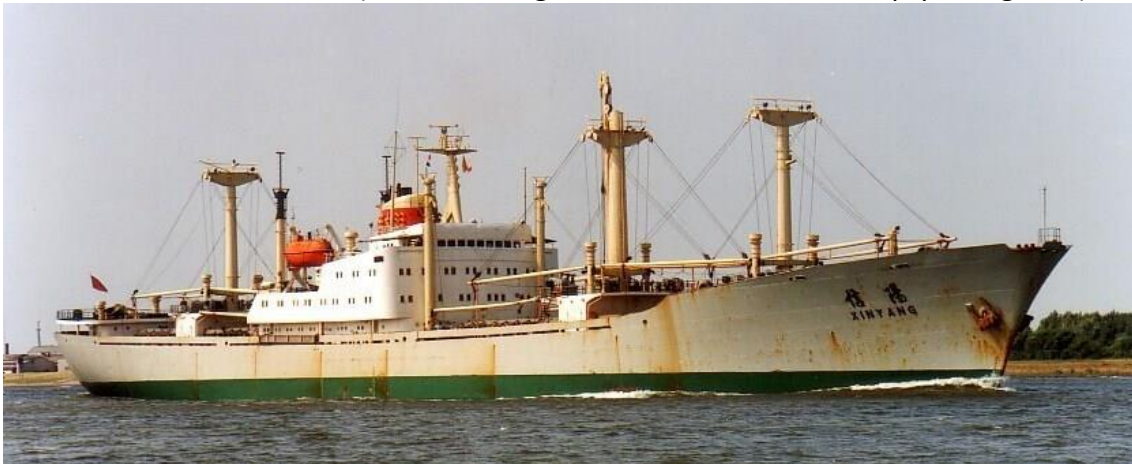
XIN YANG at Rozenburg, August 1992 retrofitted with capsule lifeboat, funnel extension and mast adjustments (Henk Kouwenoven/shipping.com).
