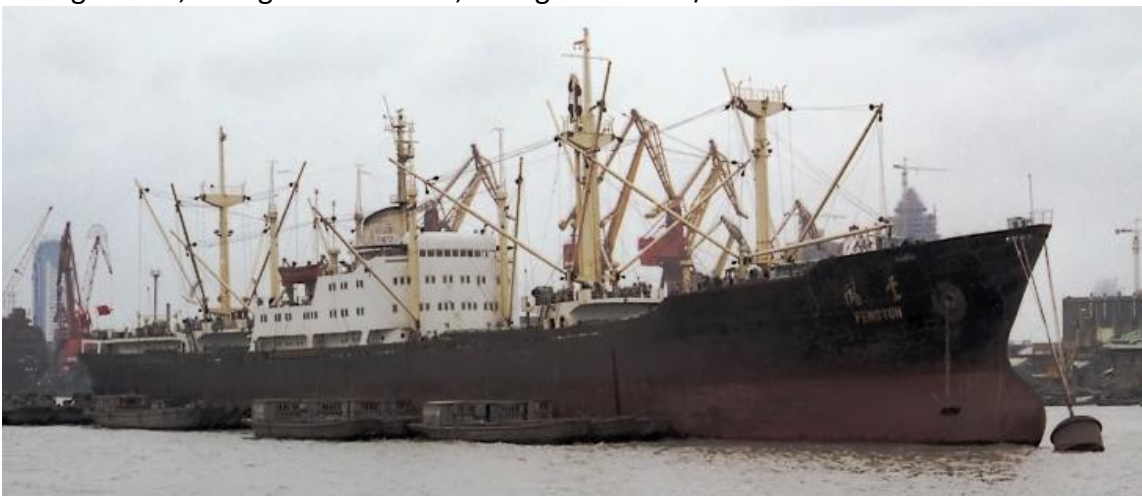
FENG YUN (March 1972) introduced the bulbous bow to the series (Markus Berger).
