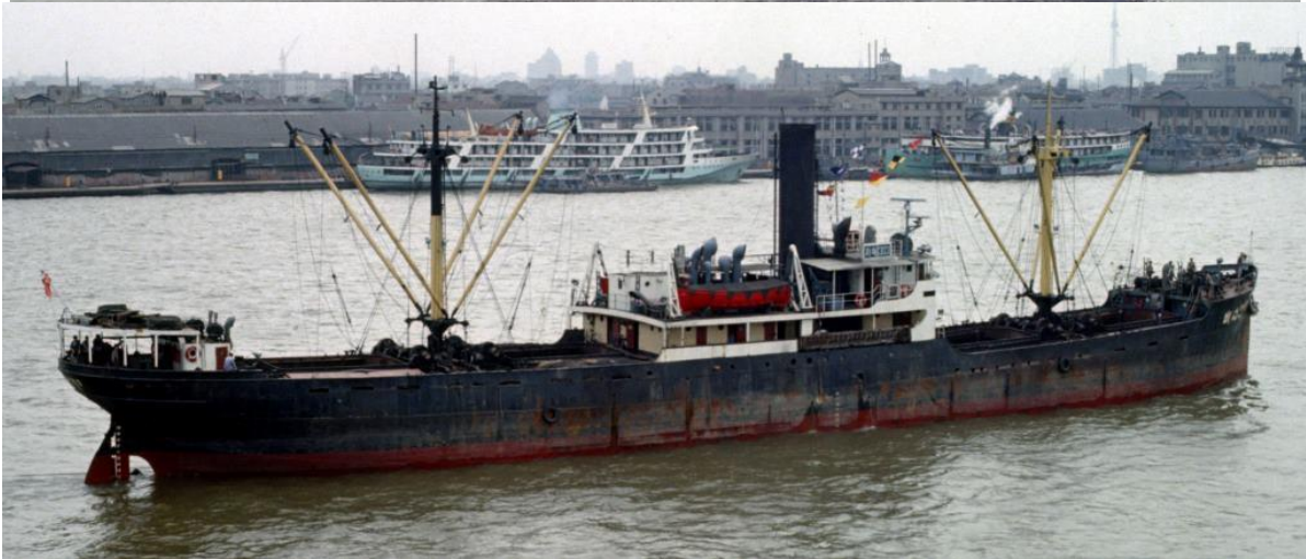
Above 3 photos ZHE HAI 303 arriving Shanghai on 18 June 1982 with new masts, superstructure plating, hull openings and portholes (Chris Mackey).
