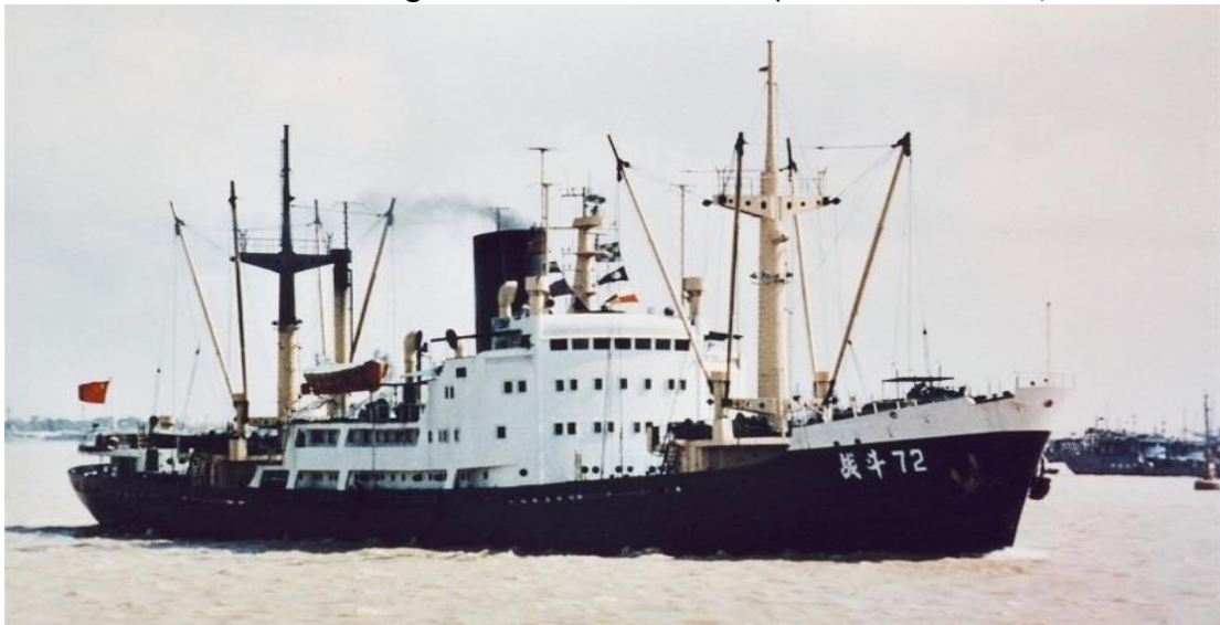
ZHANDOU 72 at Shanghai, mid-1979 (Markus Berger). 1993 RLR as ZHANDOU 72. Distinguished from Dalian-built near-sister No.77 by recognition features such as substantial radar/signal mast and absence of stanchion-like staircasing on the main deck under the bridge wings.
