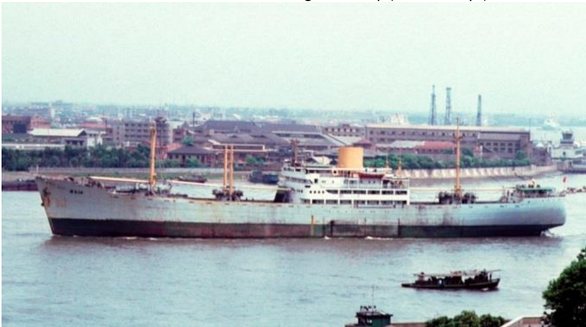
ZHANDOU 14, kingposts against superstructure removed (Jean E. Norwood in 1979/LoC coll.).
