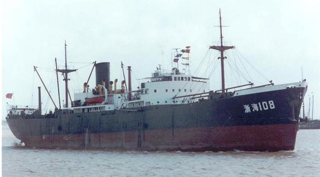
ZHE HAI 108 at Shanghai in July 1979 with plated in superstructure front for extra cabins (Markus Berger).
