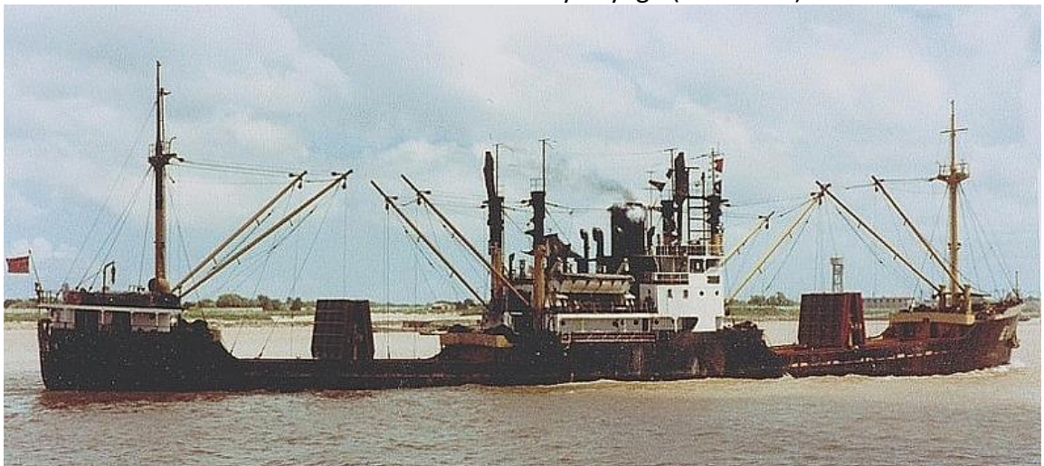
ZHANDOU 19, Shanghai July 1979, superstructure extended below bridge (Markus Berger).
