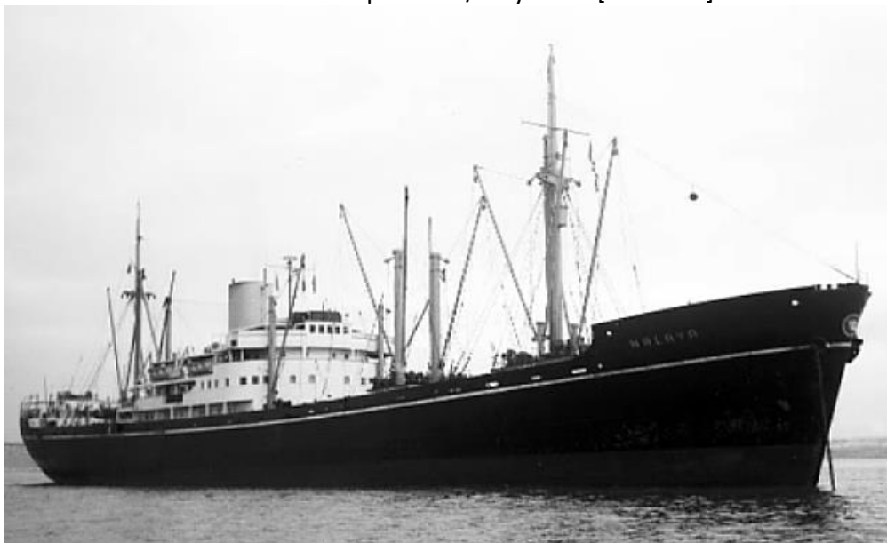
MALAYA was built with a set of kingposts against the superstructure (TORRENS/ShipsNostalgia).
