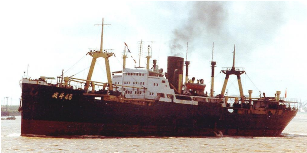
ZHANDOU 46 at Shanghai in mid-1979. The forward and aft sets of kingposts have been removed. (Markus Berger).
