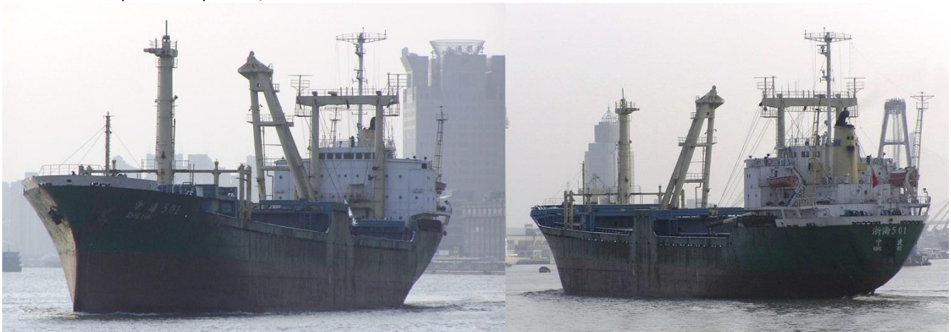
ZHE HAI 501 of Ningbo with a starboard heavy lift derrick mount in February 2005 (Hans Rosenkranz).
