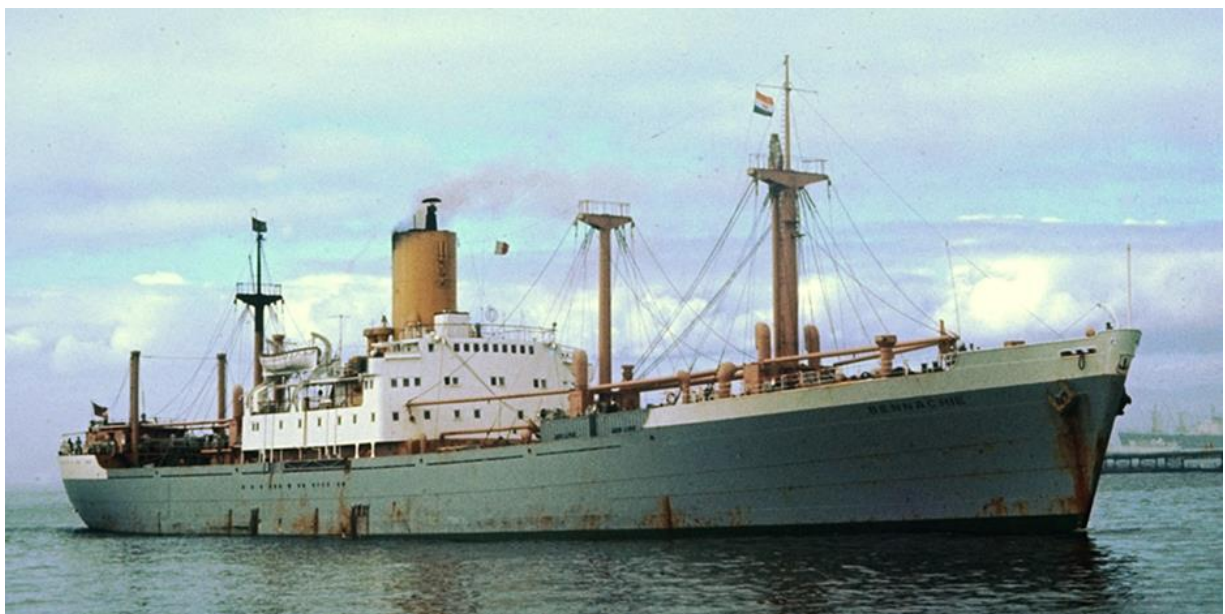
BENNACHIE with radar re-situated atop funnel (Ian Schiffman/coll. SK).
