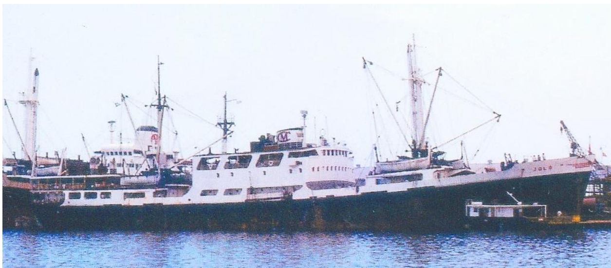
JOLO ex MUI LEE at Manila, 24 May 1970, with rebuilt foremast house, superstructure and aft accommodation for increased tween-deck passenger capacity (W. Schell*).
