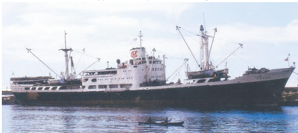
LUZON at Manila, 24 May 1970 refitted as an interisland passenger ship, built up fore, centre and aft with expanded superstructure and boats at both masts (W. Schell*).
