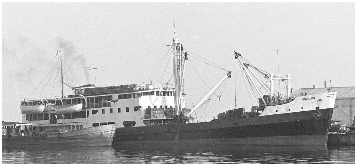
Lengthened ROMBLON with new superstructure forepart at Manila, 3 June 1970 (W. Schell).
