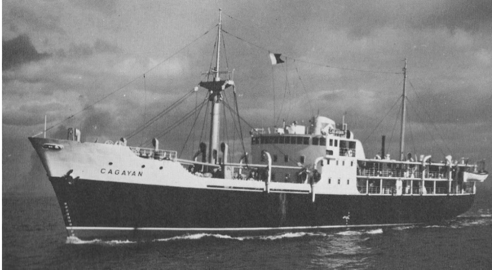
CAGAYAN on trials, Everett funnel. Pair of forward lifeboat davits later moved aft (builders).
