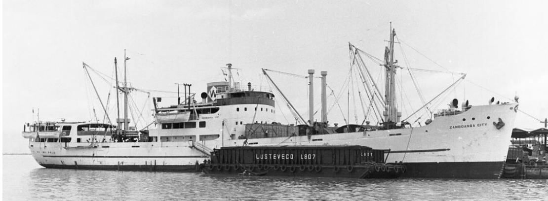
Later as ZAMBOANGA CITY at Manila, 11 June 1970. New structure at poop, six boats, extra inflatables at base of mainmast (W. Schell).
