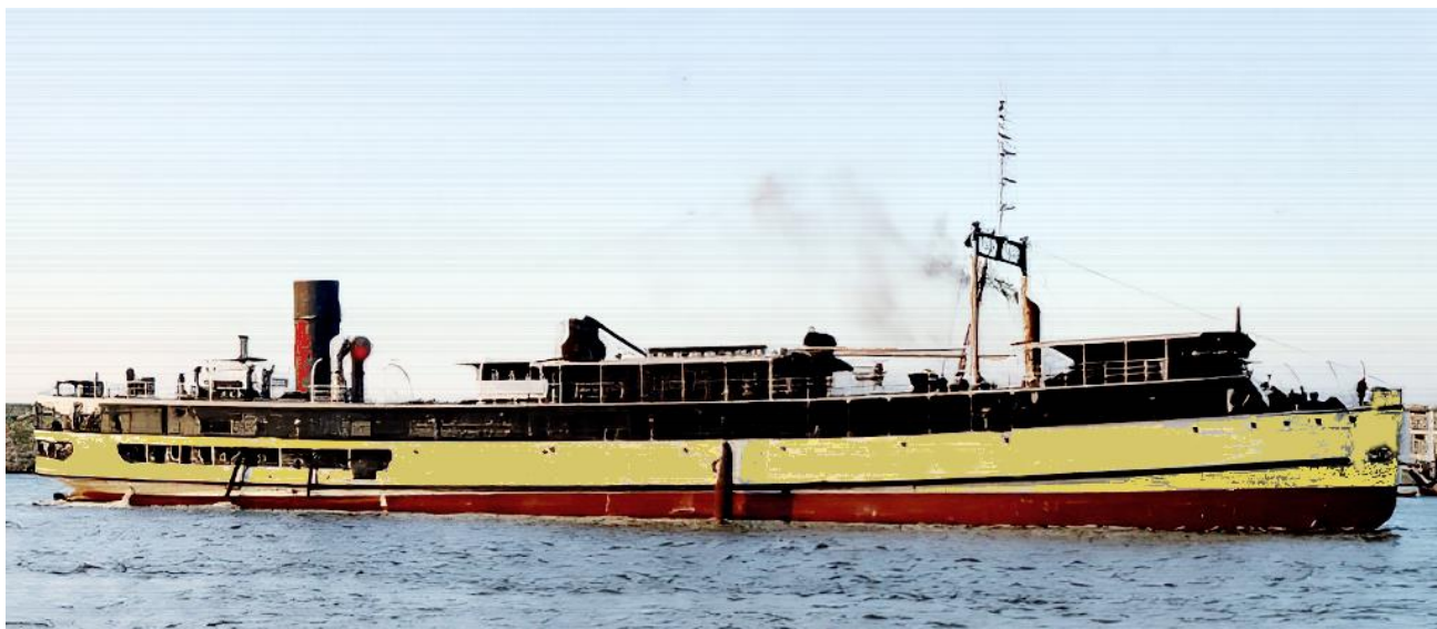
PAOWO with derricks and cranes atop superstructure (1930s coll. H. Dick per Capt. J. Pring, colorized HitPaw AI)
