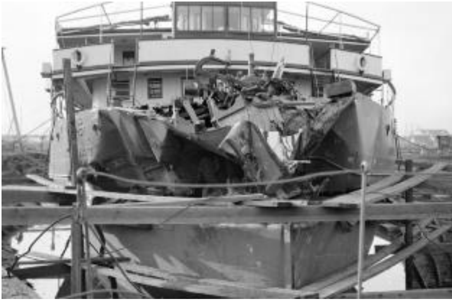
YOH YANG MARU damaged after a collision with KIANG HSIN, date unknown (Warren Swire colln).
