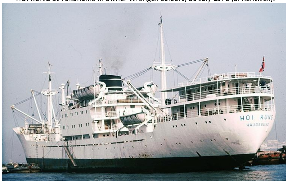
HOI KUNG Yokohama, 30 July 1973 portholes show passenger 'tween deck and crew accommodation aft (S. Kentwell).
