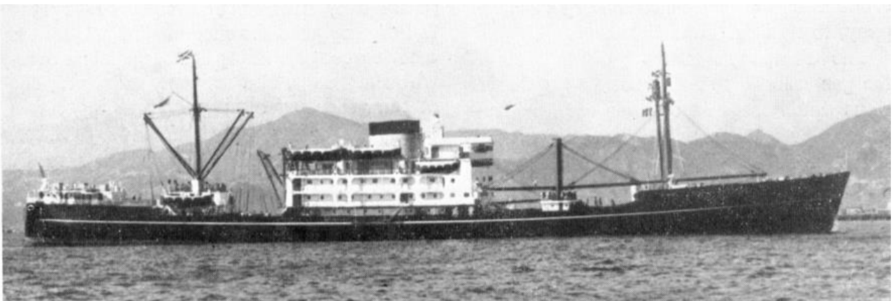
EASTERN QUEEN as originally built for the Calcutta line with squat funnel and minimal plating around the centre island (JM&C).
