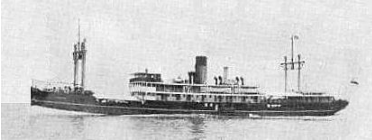
LIENSHING heavily laden, with deck awnings, canvas vent, and re-angled cowl ventilators (SK coll).
