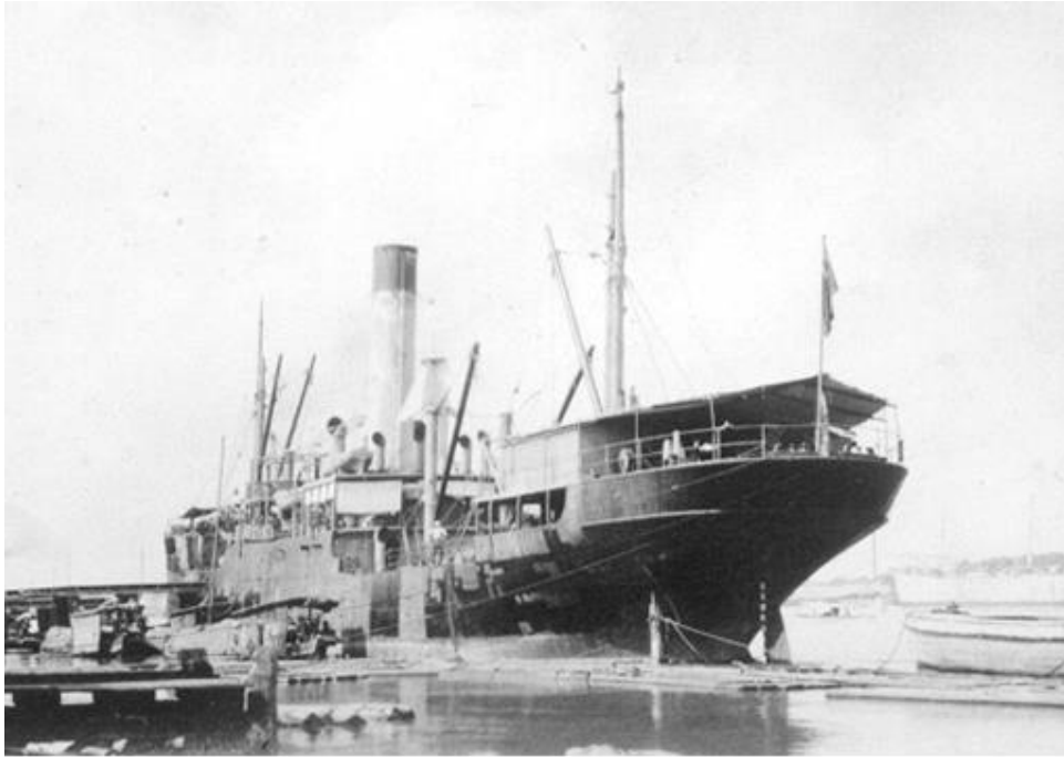
YU SANG. Built for George Shaw for China coast service. Stern housing added later (JM&C).
