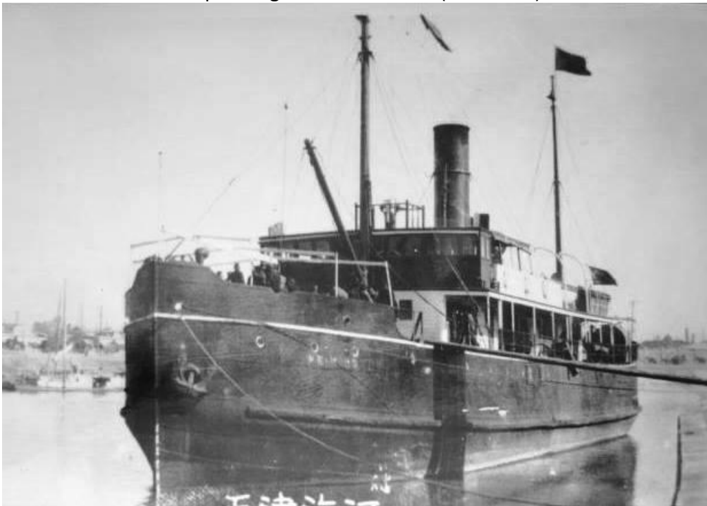
Postwar with new foc'stle & mainmast (SK*)
