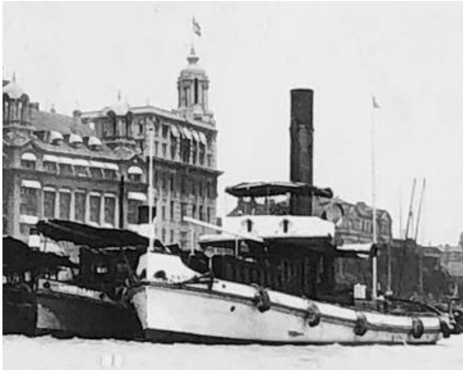
Presumed mail/passenger tender-tug SAMSON at the Bund. Enclosed passenger space beneath and forward of the bridge (Virtual Shanghai).
